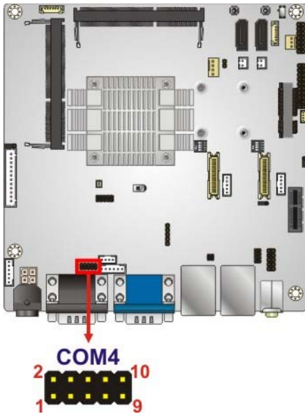
Figure 3-25: RS-232 Serial Port Connector Location
