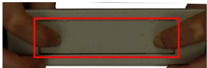
Figure 15: Bend off the front cover of the 3.5" drive bracket
