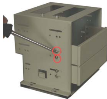
Figure 13: Remove the Front Metal Cover Retention Screws
