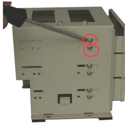
Figure 14: Remove the Four Retention Screws on the Sides of the Main Bracket
