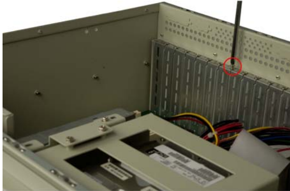
Figure 9: Remove the Slot Cover Retention Screw
