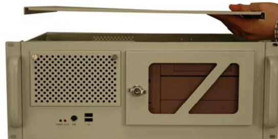
Figure 4: Remove the Top Cover
