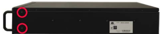
Figure 18: Insert Two Retention Screws for Each Handle
