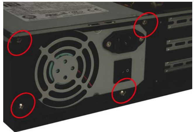
Figure 4: Insert Four PSU Retention Screws
