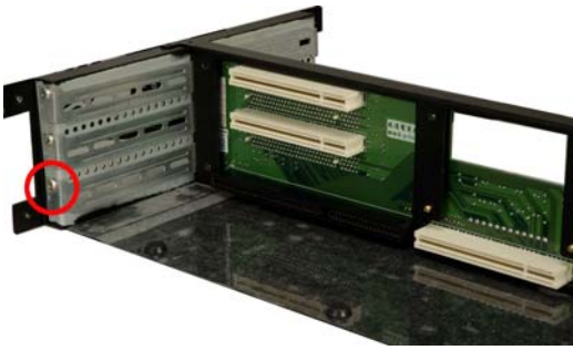
Figure 9: Remove the Slot Cover Retention Screw
