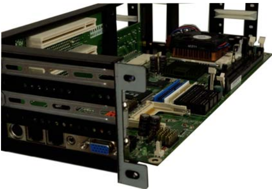
Figure 10: Secure the CPU Card to the Backplane Bracket
