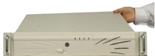
Figure 5: Remove the Top Cover
