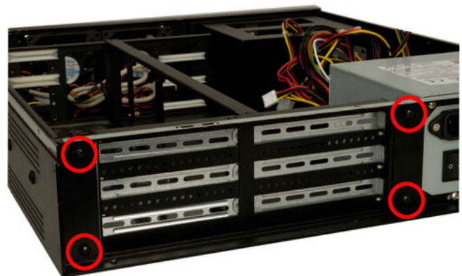
Figure 16: Four Backplane Bracket Retention Screws at the Rear of the Chassis
