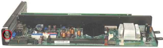
Figure 21: Secure the CPU Card to the Backplane Bracket
