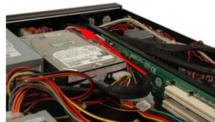
Figure 31: Run the Ribbon Cables through the Space between the Backplane and the HDD
