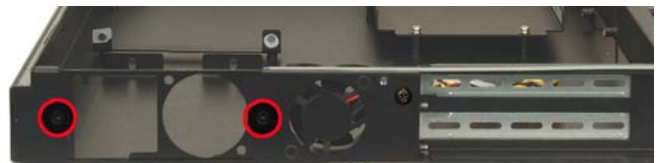
Figure 5: PSU Bracket Retention Screws at the Rear
