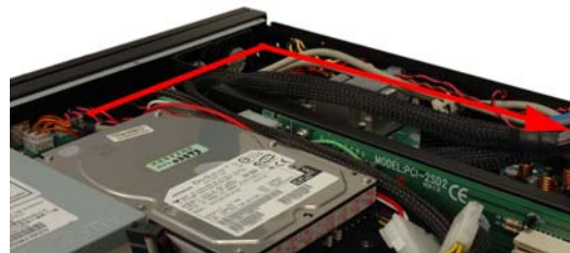
Figure 33: Run the LED, USB, Power and Reset Cables along the Right Side of the Chassis
