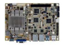
NANO-BT-i1 — This EPIC computer supports dual independent displays with LVDS, VGA, and HDMI. It also supports IPMI 2.0 with iRIS-1010 module, and features IEI one key recovery solutions, allowing customers to create rapid OS backup and recovery.
